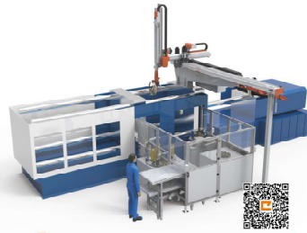
引擎冷却风扇模内插入注塑自动化系统 In molding Inserting Molding Automatic System For Cooling Van On Automobile Engine
